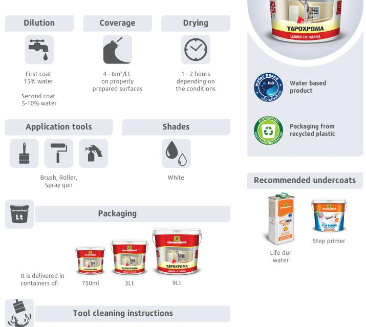
Keep the tools "wet" in the container during work. Drain the product thoroughly from the tools and clean them immediately with warm water and soap. If the product dries out, clean only with strong detergents. Do not empty washing liquids into the water table.
